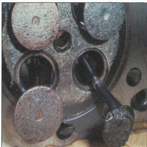
Carbon build-up on inlet valves
