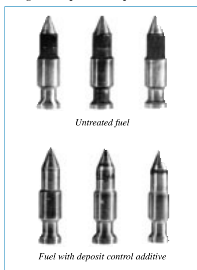
Figure 7-2 Typical Deposit Levels on a Fuel Injector Plunger Susceptible to Deposit Formation
